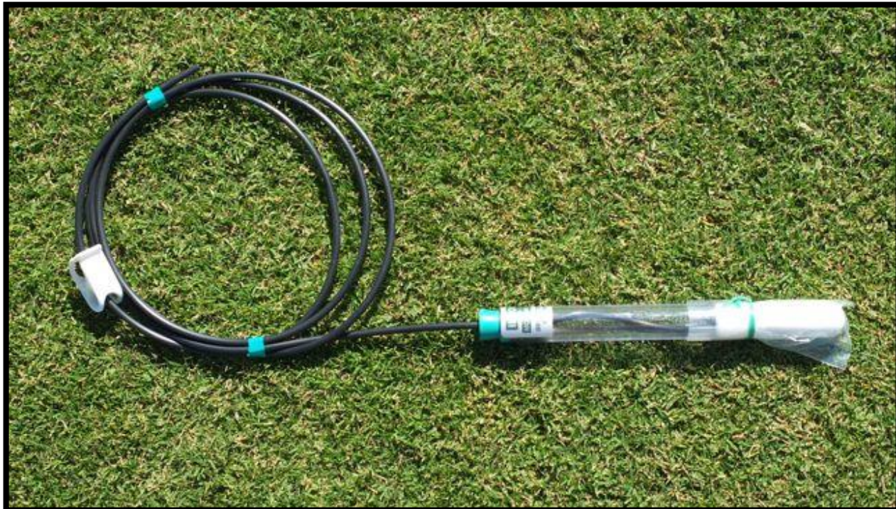
Figure 1. Suction lysimeters (Irrrometer, Riverside, CA) used to capture leachate for analysis of EC_L . Lysimeters were buried 4 inches below the turf surface in 3 out of 6 replicate plots for each treatment.
